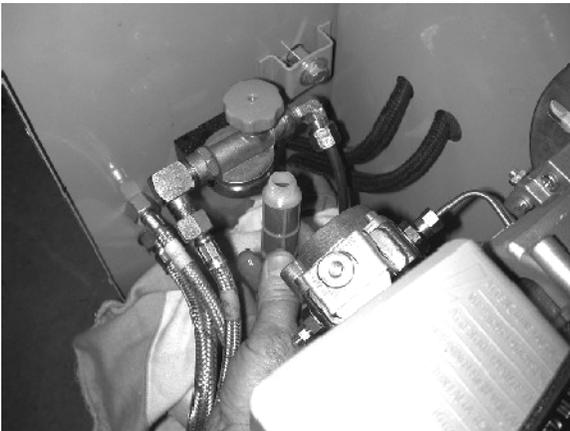
Unscrew the fuel intake filter by hand
