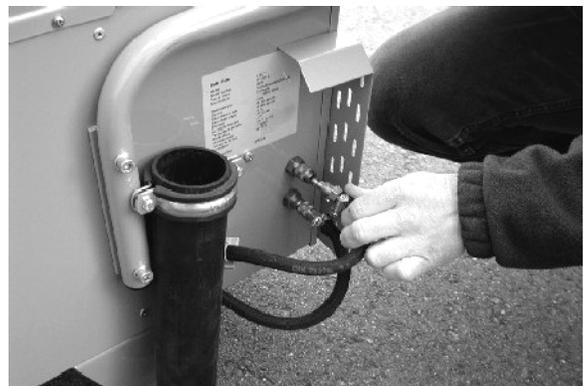
Connect the internal tank fuel lines
