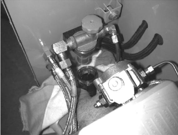
Unscrew the filter reservoir by hand
