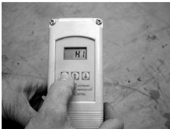
**Important!** Make sure the thermostat is set to H1 for the heating mode. The Dragon will not function properly with the thermostat in cooling mode.
