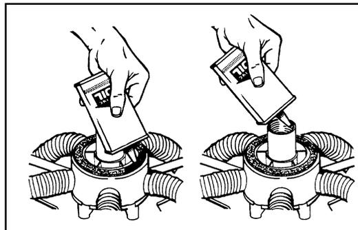
9. Coat the shaft with Pennz-Guard or a similar lubricant. Reinstall the vacuum head assembly onto the shaft by rotating it counter-clockwise.
