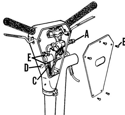
1. Remove the 440 male quick connect (A) with a wrench.
