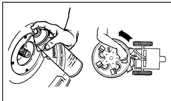
**IMPORTANT:** While rotating the vacuum head assembly in the counter-clockwise position, make sure that it spins freely all the way down. If it begins to require the slightest finger tip pressure, unscrew it and brush off the threads. All it takes is the slightest grain of dirt or sand to obstruct the threads. If you turn too far onto a grain of dirt, the hub may become locked onto the shaft of the gearbox.
