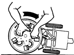
To prevent the gearbox from turning, the output shaft will accept a 5/8 inch wrench just below the rotary union. Wash the cleaning heads and shroud assembly with a garden hose, being careful not to wet the electric motor assembly. Clean any lint buildup from the cleaning heads and vacuum hoses (lint buildup will restrict proper airflow and prolong drying time).
