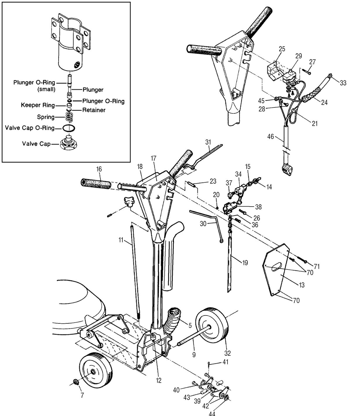
Figure 2 High Speed Base Assembly
