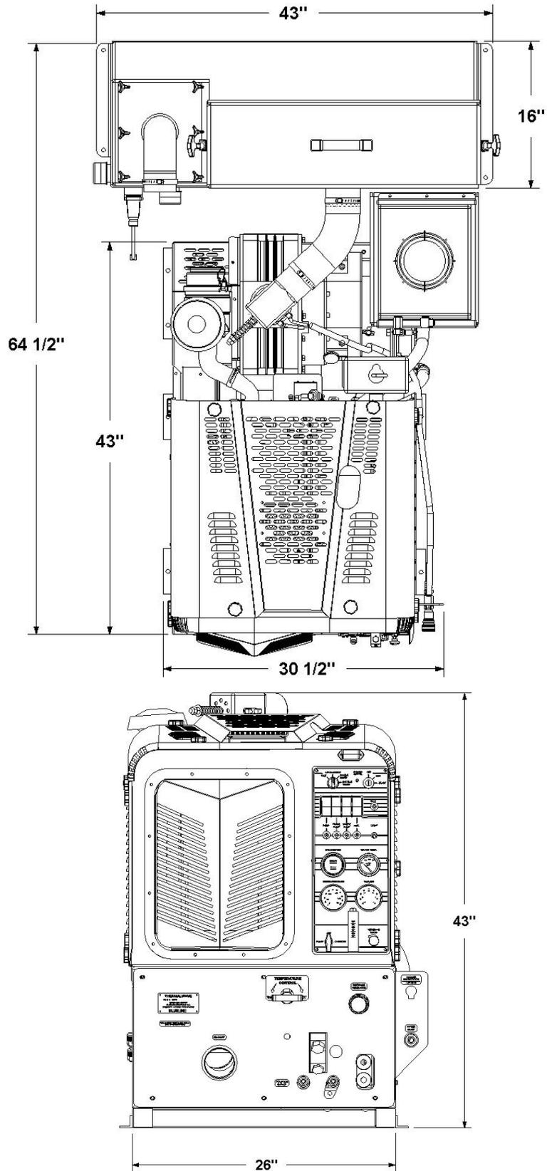
**DIMENSIONAL DIAGRAM w/ SUB-MOUNT WATER TANK**
